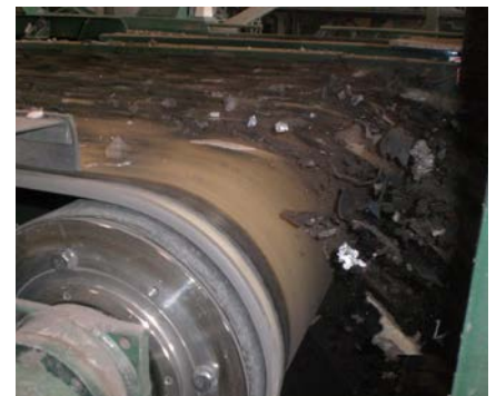
Breda 22UF-TR , magnetic separator.
