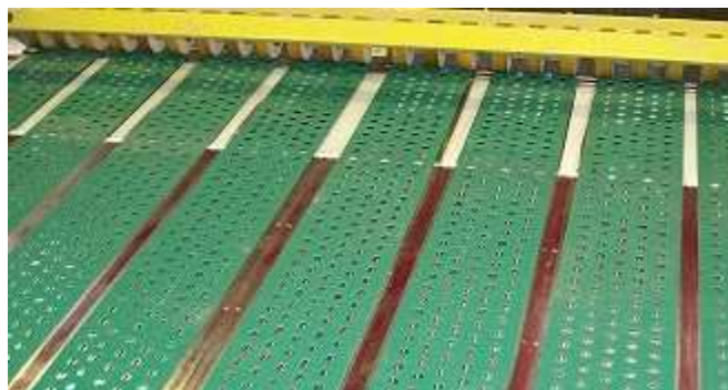
Perforated belt for the corrugated carton industry.
