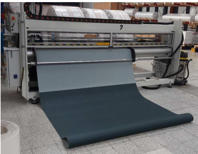
Belt on the punching machine ready to be perforated.
