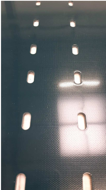
Slotted holes measuring 16 x 7mm.
