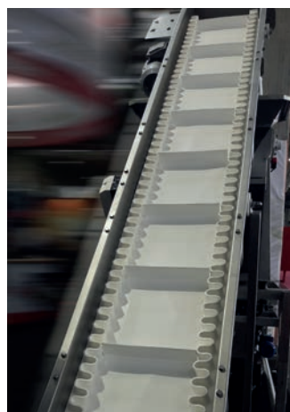
Conveyor belt with cleats and sidewalls "Runer".
