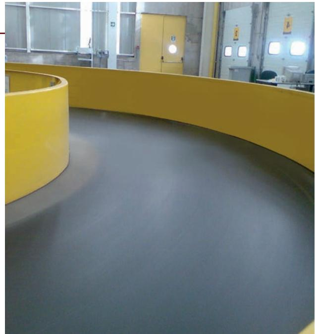
■ **esbelt** has developed a range of belts for these applications. These belts need to be flexible, strong, stable and able to withstand significant flex fatigue due to the unconventional flexing the belt undergoes during operation.
