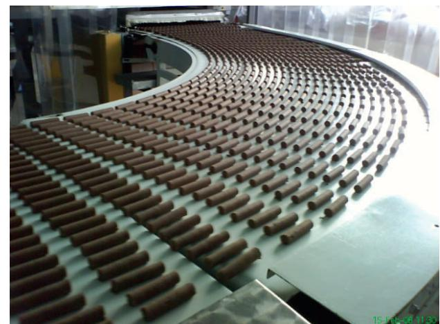
■ **esbelt** manufactures Power Curve belting in 3000 mm (118") width and through experience can provide many belts with one splice maximizing fabrication quality and belt performance. When Spirals and specialized belts require multiple splices the esbelt system and belt materials deliver the required reliability through consistent materials and fabrication performance.
